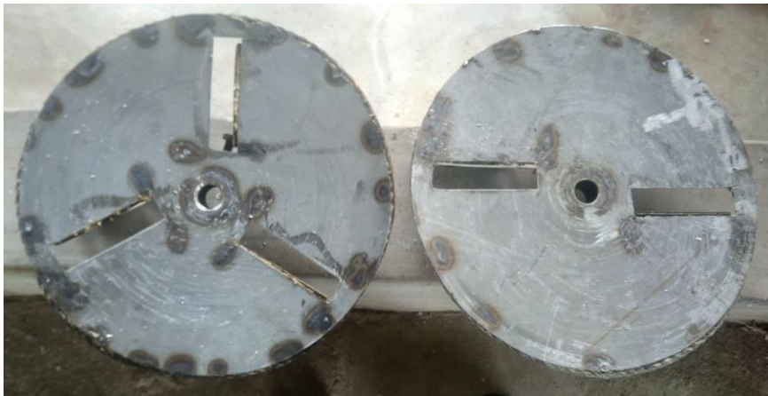
Plate 2. Three and two blade chipping discs.
