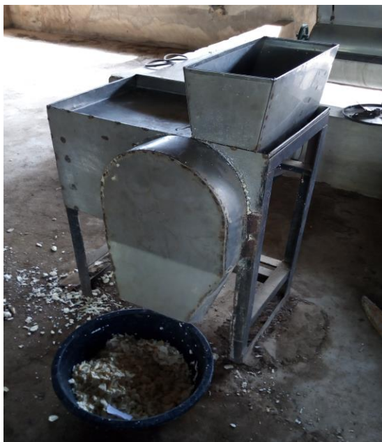
Plate 4. Cassava chipping machine in operation.
