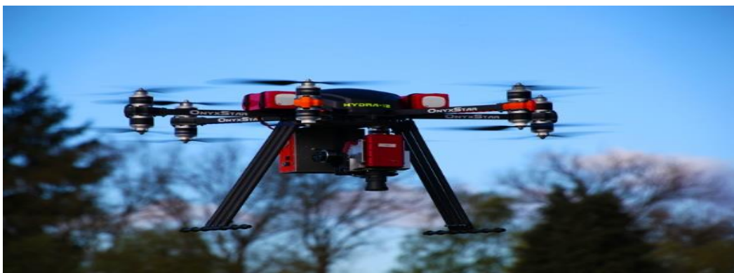
A hyperspectral camera embedded on OnyxStar HYDRA-12 UAV from AltiGator
