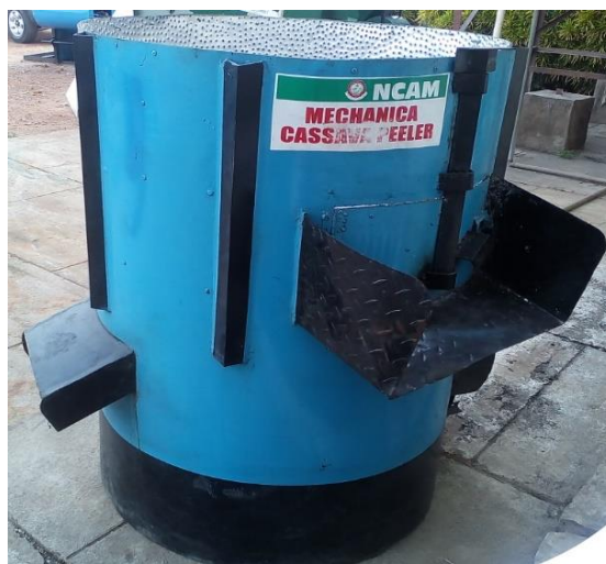
Plate 1: Pictorial view of the motorized Rotary Cassava peeling machine.
